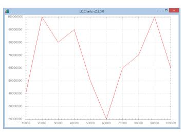
If you use the **/nomag** option or set **xMagAuto** to **0**, you can still format the X-Axis and Y-Axis labels easily to not display all the zeroes (see the xXAxisFormat, xYAxisFormat and xY2AxisFormat properties)
