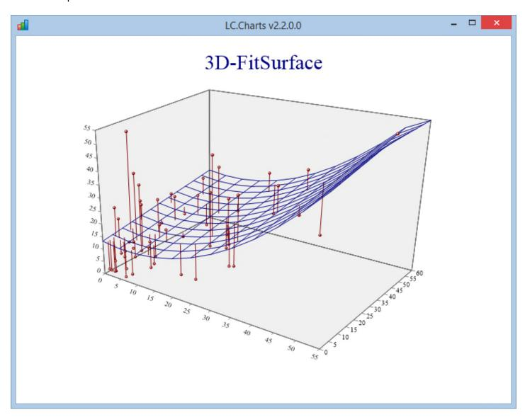
In LC.Charts v2.2.0.0, the model is quadratic on the X and linear on the Y values.
